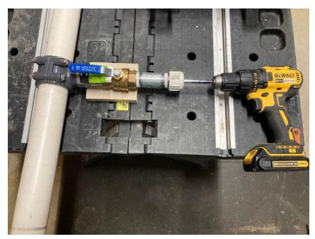
With the ball valve fully open, the hole saw is extended until it makes contact with the wall of the water distribution main. The drill powers the hole saw to provide a  $\frac{3}{4}$ " hole (tap in) in the wall of the pipe. The assembly is then retracted back through the open ball valve into the galvanized pipe nipple. The ball valve can then be closed isolating the water
